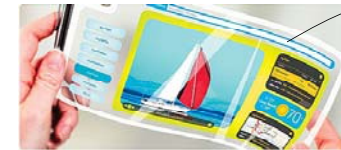
4" flexible transparent OLED from University Display and LG
