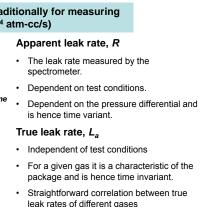
Typically, the apparent leak rate has been used as a hermeticity metric. For small volumes, this can produce erroneous results.
