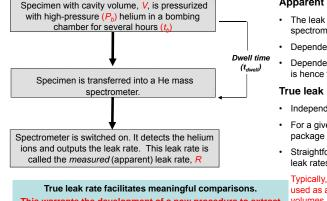
This warrants the development of a new procedure to extract the true leak rate from the helium leak test data.
