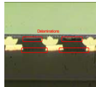
Delamination of underfill by hygroscopic swelling and adhesion degradation
