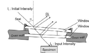
Optimization of beam polarization with respect to the plane of incidence.
