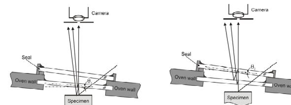
Window angle optimization to eliminate undesired interface patterns
